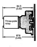
Note: Model PF113A-E can be used as a front connecting socket.
